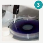
As the agar plate spins, the syringe automatically dispenses accurate volumes of sample over the plate drawing a spiral with the loaded sample.
