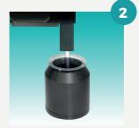
The syringe takes the liquid sample from an irradiated sample beaker.
