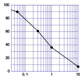
This test kit has a wide detection range between  $0.05\mu g/L$  and  $10\mu g/L$ . Samples within this range can be directly applied to the assay only after filtration.
