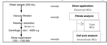
Scheme procedure for water samples from reservoirs, rivers, etc.
