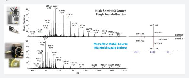
Ion-Pairing RP-LC/MS Analysis of 75-mer tRNA using the MnESI-MS platform with M3 Emitter at microflow. MnESI platform attains improved sensitivity and higher charge state and comparable data quality vs. high-flow LC/MS method.
