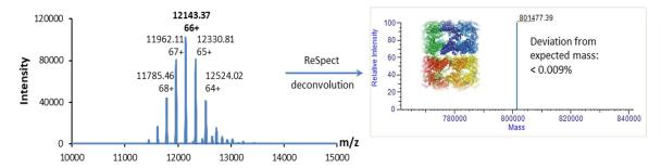
SEC-LC/MS analysis of GroEL tetradecamer protein complex using the MnESI-MS platform with M3 Emitter at the microflow of 5 μL/min.
